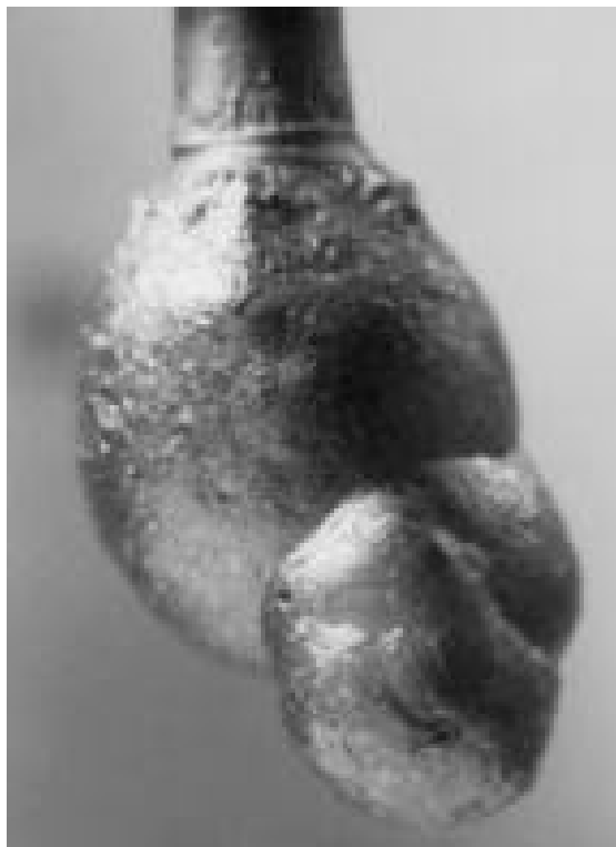
FIG. 7—Attached droplet quenched by cessation of oxygen flow, exhibiting lobes due to "extrusion" of liquid (same specimen as that of Figure 6).
